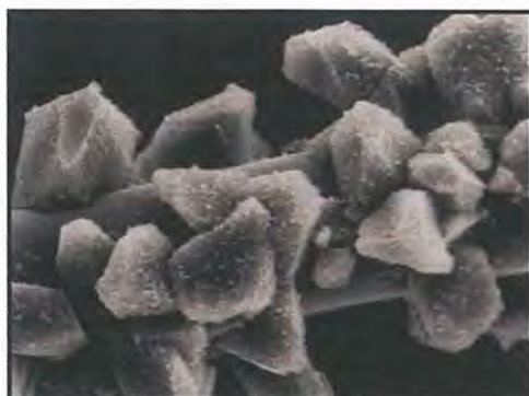
Figure 3. Cement soil stabilization – low crystal interlocking connectivity.
