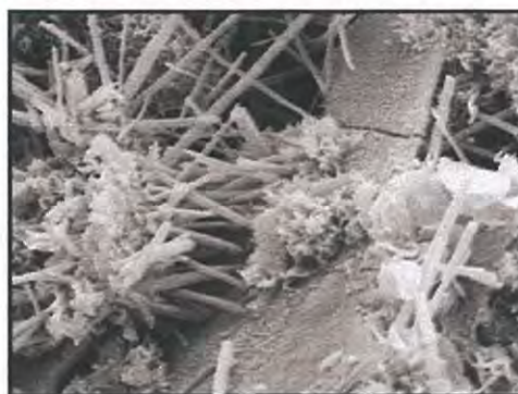
Figure 4. Cement-Geocrete soil stabilization - high crystal interlocking connectivity.
